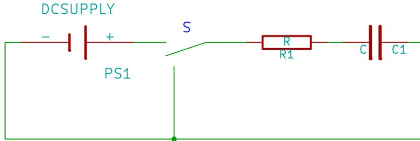
Figure 1: The switching circuit used to discuss charging and discharging a capacitor.
