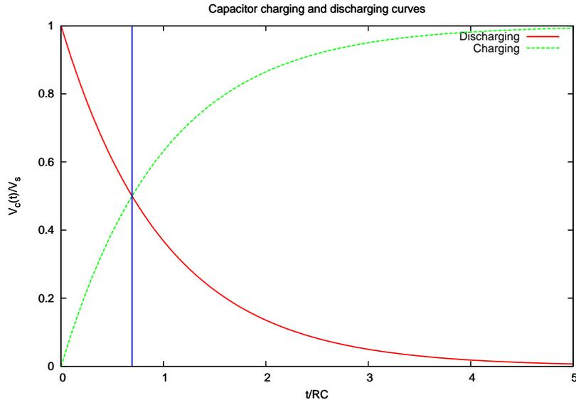
Figure 2: The capacitor charging and discharging curves. The vertical blue line is the “half life” point of the charging and discharging timeline.
