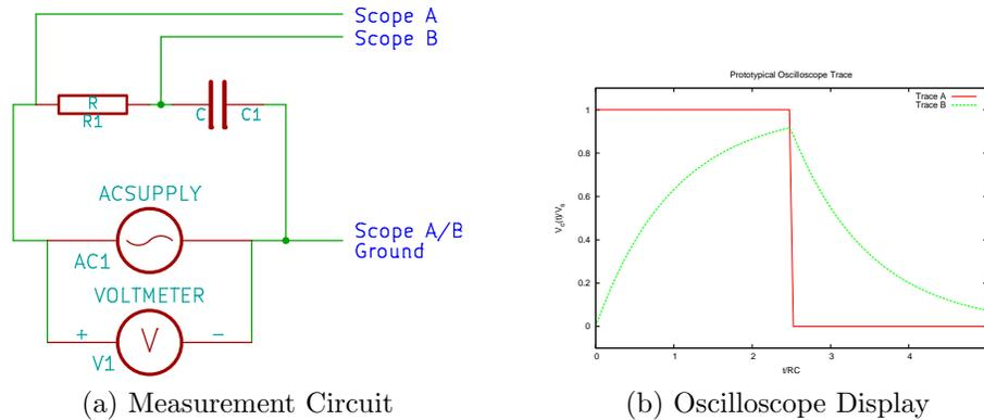
Figure 3: The left-hand figure is the circuit used to measure the time constant of an RC circuit, while the right-hand figure shows the Oscilloscope traces.
